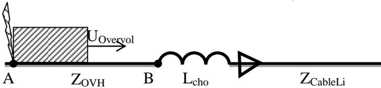
Fig. 1. Network layout with the choke
