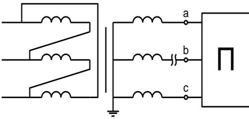
A symmetrical three-phase resistive receiver which phases are connected in a "triangle" is connected to the secondary winding of the transformer ( $\Delta/Y$ ) 6,0/0,38 kV.  $P_{\text{receiver}}=6$  kW.
