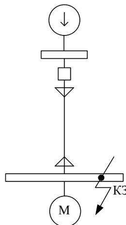
Fig. 1. The scheme of power plant power distribution
